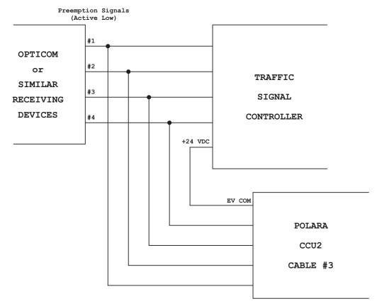
Example of Four-Way Emergency Vehicle Message Wiring
